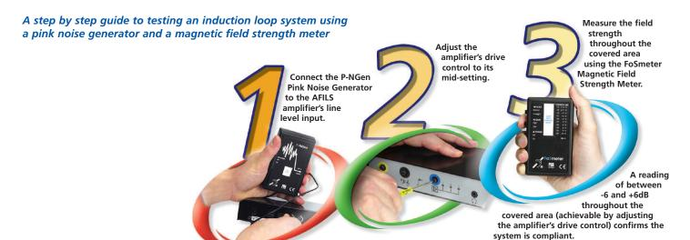
Important: Once you have verified the magnetic field strength of the system, we recommend you listen to the system's real audio source(s) using a loop listening device (such as the FoSmeter H) to ensure there is no 'clipping' or distortion. If any adjustments need to be made to the amplifier's settings, be sure to re-test the system using the P-NGen pink noise generator and a FoSmeter variant before signing the installation off.
