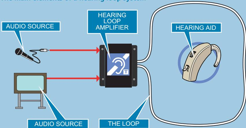
Some hearing loop systems may require additional audio sources such as multiple microphone or line level inputs. To facilitate this, many PDA range amplifiers include a patented 'Outreach' socket which allows the connection of multiple inputs via a range of specially designed single gang audio connector plates. This system is described in detail on page 26.
