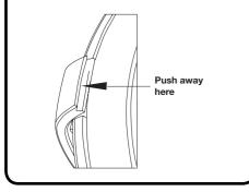
To fit the neck cord remove belt clip and thread the cord as shown, and replace the belt clip. The neck cord has a safety release feature to avoid you getting trapped by the cord.
